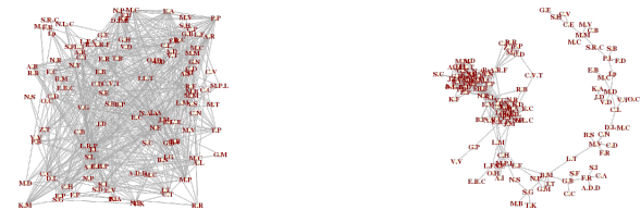
FIGURE 4 – My facebook network displayed with a random layout (left) and with a layout produced by a force-directed placement algorithm [Fruchterman and Reingold, 1991] (right).
